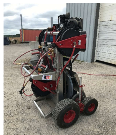
Figure 14: Mobile Strapping Station
