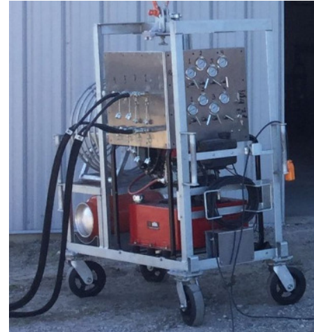
Figure 10: 10,000 PSI Synchronized Power Unit
